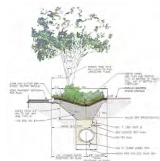
Bioswales are landscape elements designed to remove silt and pollution from surface runoff water.
