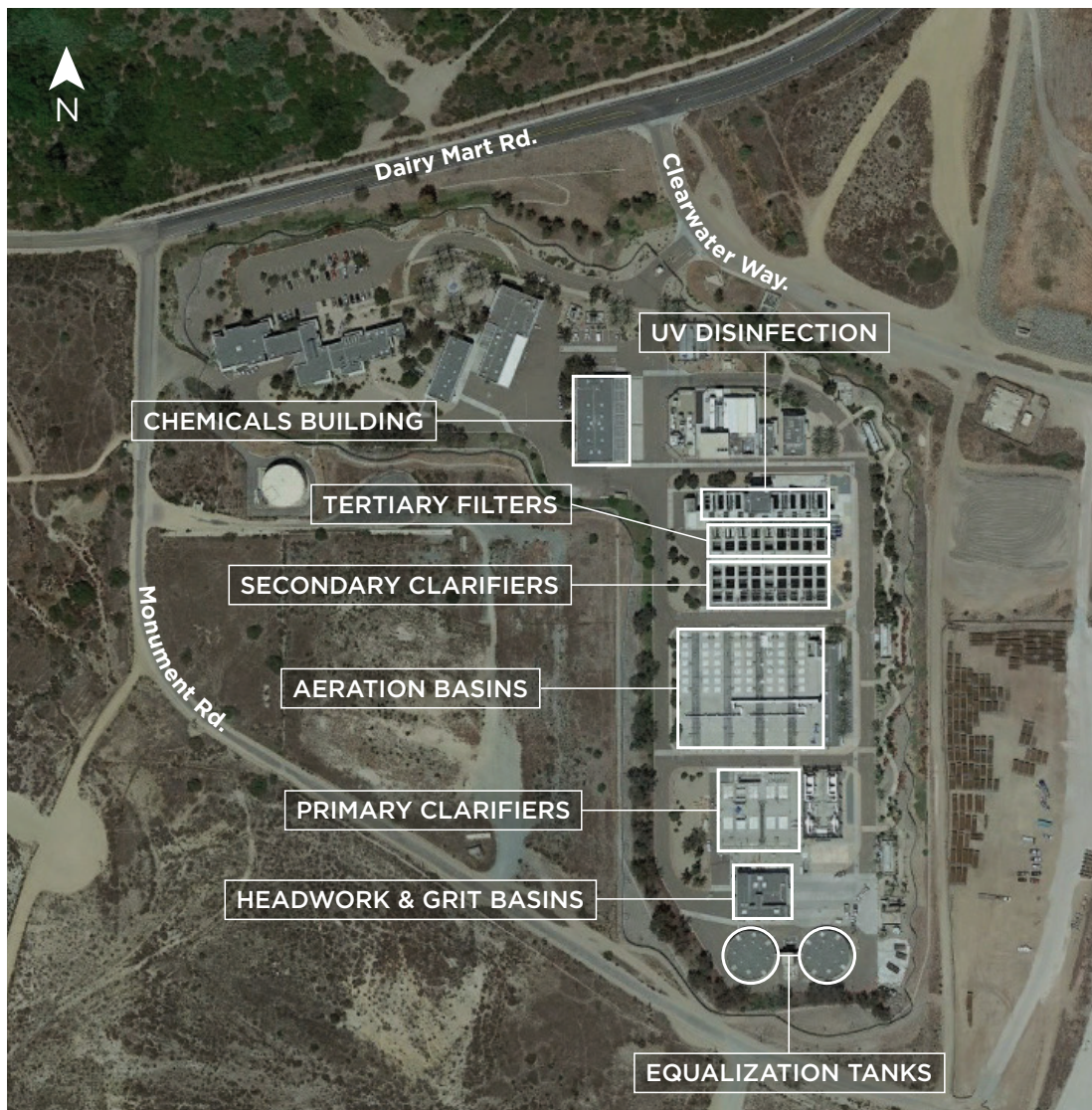
Figure 4: Layout of South Bay Water Reclamation Plant
