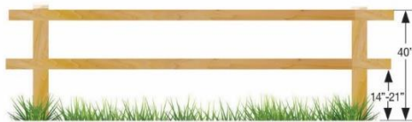
Figure 29. Posts should not extend beyond the rails making it easier and safer for wildlife to jump over.
